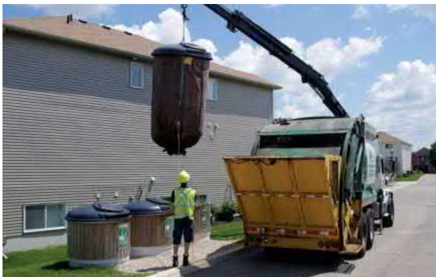
Figure 20: Waste collection for Molok underground bins
